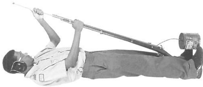
Clean the breech and barrel of your percussion model by using a flush-out nipple.
